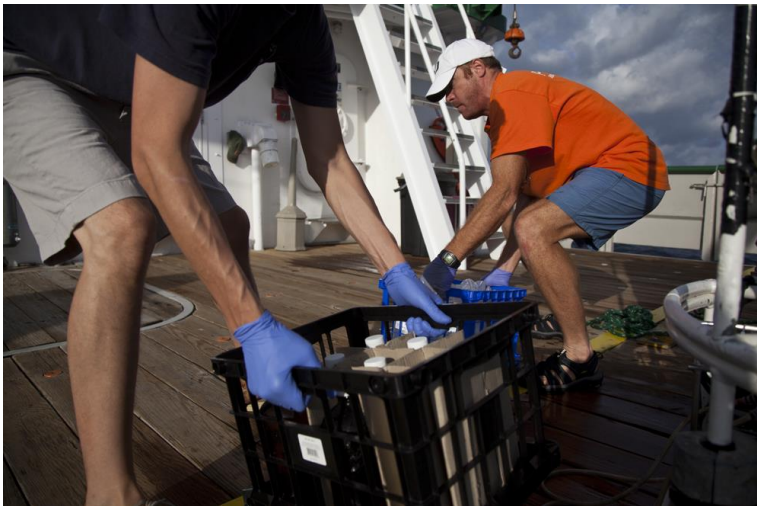
Image 1. CTD/Rosette deep water cast. Seawater samples were collected in 1 liter glass bottles. (FIO-BP R/V Walton Smith Cruise; Oct 3-13, 2011; photo credit: Marlena Skrobe).
