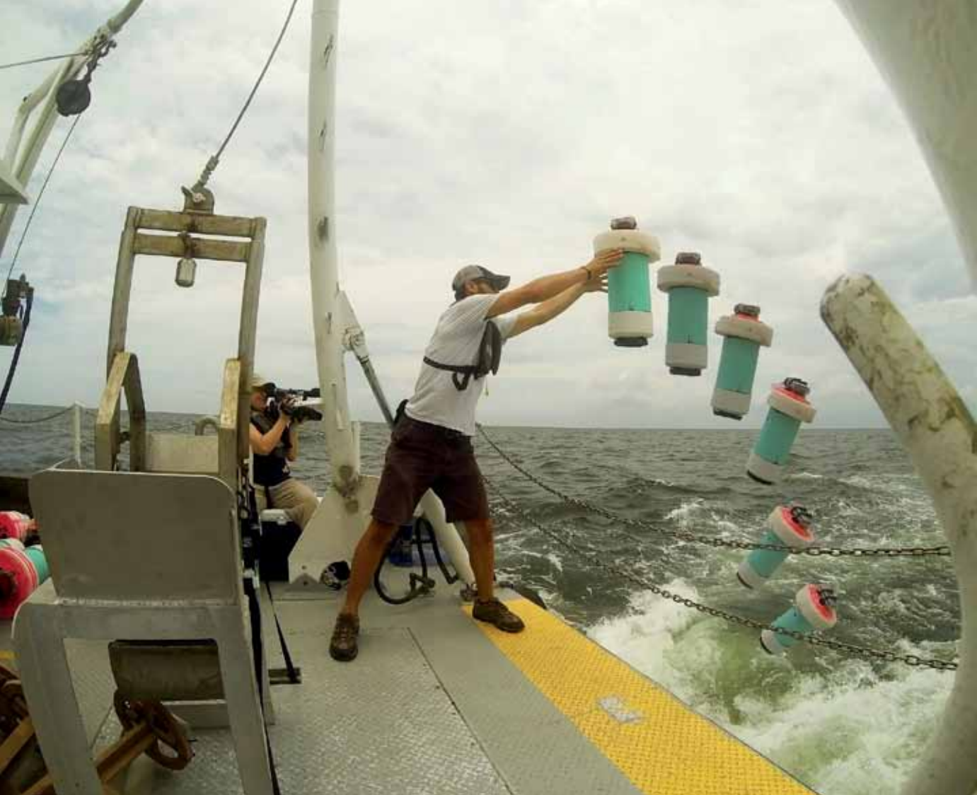
In this time lapse photo, CARTHE member Conor Smith deploys a GPS drifter, which sends accurate surface flow data to modelers and responders. Photo: CARTHE.
