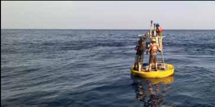
60 miles offshore and clinging to a buoy, it's not a survivor story but a maintenance call. A USF team preps a buoy swap by removing instruments before its pulled onto the R/V Weatherbird II and replaced with a new mooring. Credit: Mark Collins.
