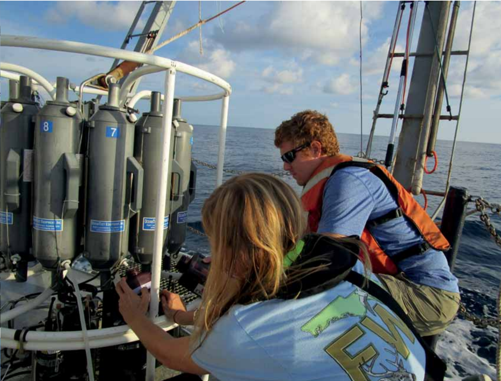
Above: Each sampling bottle traps water at a specific depth in the water column. Here, Research Scientist Kate Hubbard and Technician Eric Muhlbach are filling smaller bottles with water from deep in the Gulf. Opposite, top: Either collecting data on the way out or processing it coming back, passing the Skyway on the R/V Bellows always means more work ahead. Opposite, bottom: HAB researchers smile. Photos: FWC.
